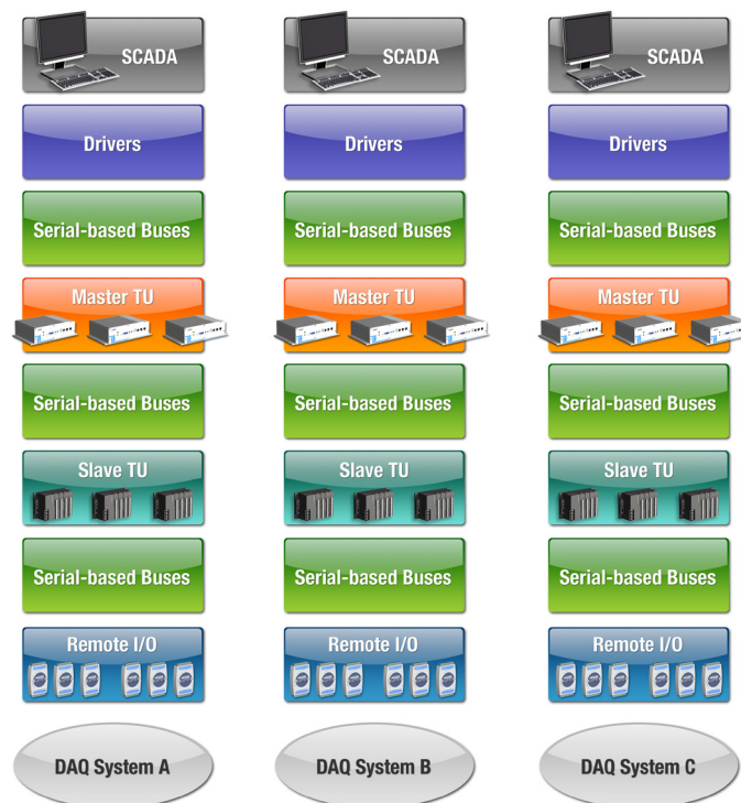
A system with too many data acquisition layers is costly and time-consuming to deploy and maintain
